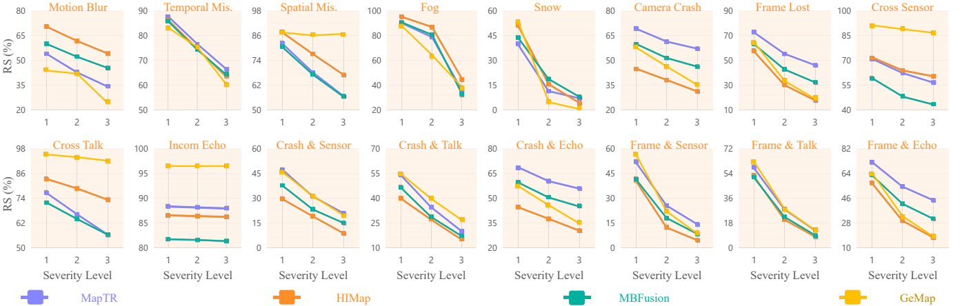
Fig. 4. Robustness against all corruption types and severity levels in HD map construction tasks is assessed using the Resilience Score (RS), calculated based on the mAP score for different severity levels.
